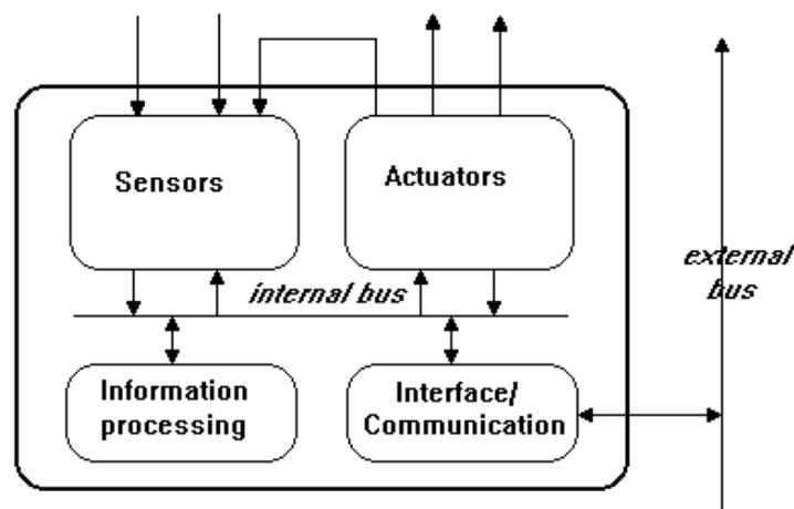
Figure 1. Example of Microsystem Architecture (Source IMT Karlsruhe)
