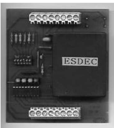
Fig.7 PCB-construction, PCB for WEB case M 1 : 1 size 85x95
